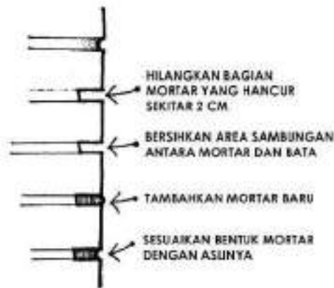
Gambar II. 2 Cara melakukan Repointing
